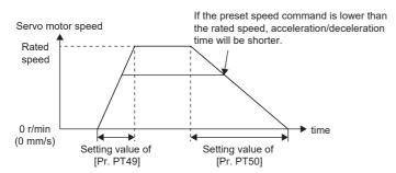
For example, for a servo motor with a rated speed of 3000 [r/min], set 3000 [ms] to accelerate from 0 [r/min] to 1000 [r/min] in 1000 [ms].
