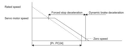
This servo parameter corresponds to [Quick stop deceleration (Obj. 6085h)]. When the object is mapped to the cyclic communication, do not write values with engineering tools because the controller overwrites the servo parameter values written with engineering tools.
