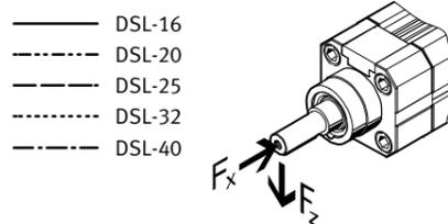
The mass moment of inertia of the moveable mass should be calculated. Lever arms, jibs and masses, as well as masses on the square must be taken into consideration in the calculation.
