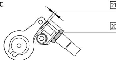
3. Screw the shock absorber into or out of the shock absorber retainer using a hexagon spanner. The permissible unscrewing lengths are summarised in the following table.
