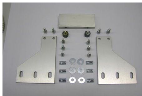
Fig. 24 Individual parts of the stroke limitation
