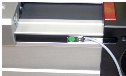
Fig. 5 Portal axis with mounted reference sensor
