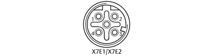
Fig. 4-3 Fieldbus connection pin assignments
