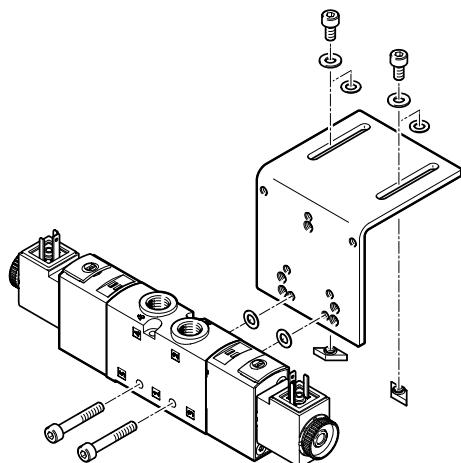
For mounting individual valves directly on a drive.
