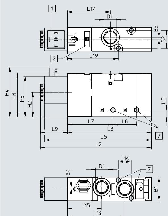
[1] Solenoid coil interface type B/
