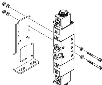
For mounting individual valves on a flat surface, e.g. aluminium profile systems.
