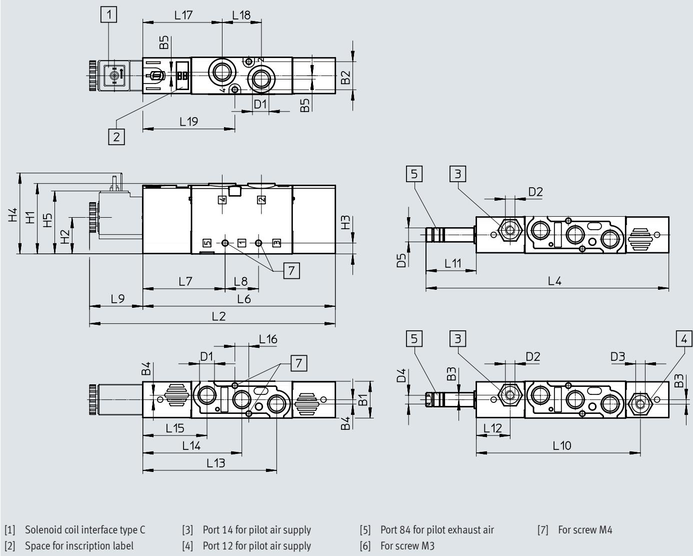
[1] Solenoid coil interface type C
