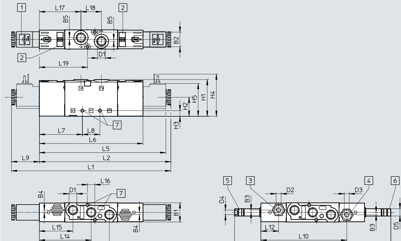
[1] Solenoid coil interface type C
