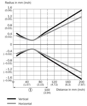
① Minimum distance between sensor and reflector
