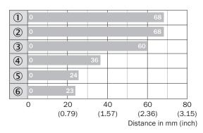
Max. sensing range S<sub>n</sub>, flush or non-flush installation, non-magnetizable material
