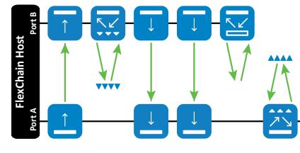
FlexChain, the individual light grid: Whether through-beam photoelectric sensors, photoelectric retro-reflective sensors or photoelectric proximity sensors – the sensor technology can be freely selected and combined.
