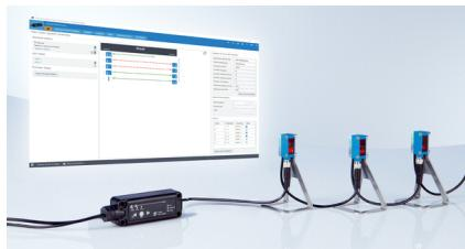
Intuitive operation: Define zones, configure logic, and monitor the sensors with ease using the SOPAS software tool – convenient connection of the FlexChain host via USB
