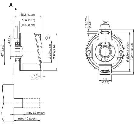
$\bigcirc$  Cable diameter = 5.6 mm +/- 0.2 mm bend radius = 30 mm
