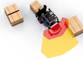
The use of two sensors is also recommended in environments with complex travel paths in order to provide optimal protection for lateral areas.
