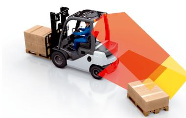
A system variant with two sensors is well suited for targeted coverage of blind spots.
