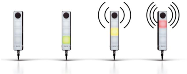
The signal light bar supports the driver with visual alarms. Green means clear travel path. If an object is detected in warning field 1, the color changes to yellow; if it enters warning field 2, it changes to red. Depending on the monitored area, the lamp emits additional acoustic warning signals via an integrated up to 98 dB buzzer.
