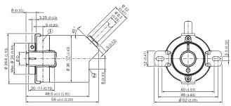
Non-tolerated dimensions according to DIN-ISO 2768-mk ① Measuring point for operating temperature ② Measuring point for vibrations
