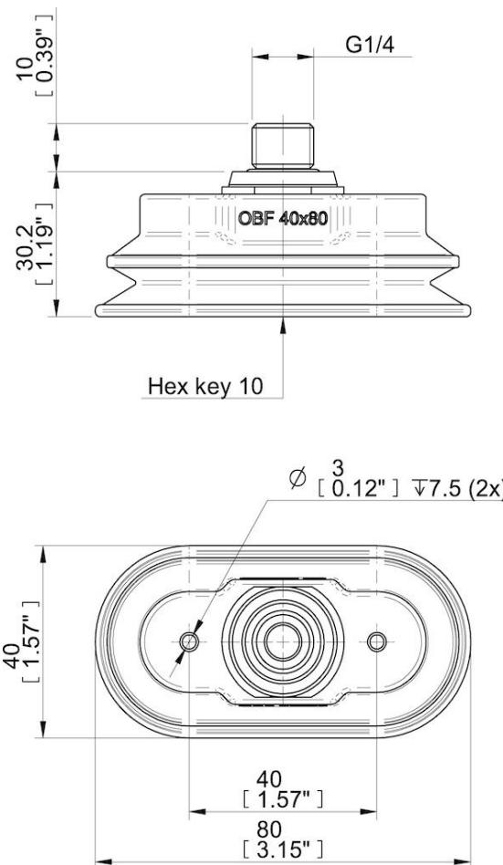
Values specified in this data sheet are tested at (unless otherwise stated):
