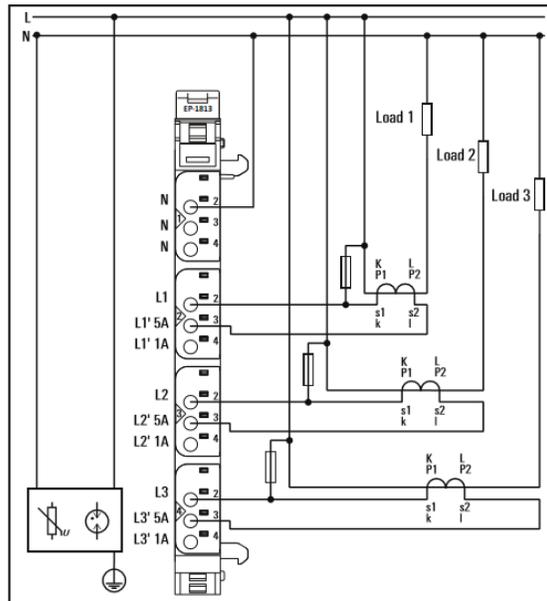
**Note:** If the module is used in an environment of overvoltage category III, transient overvoltage must be limited to  $\leq 2500V$
