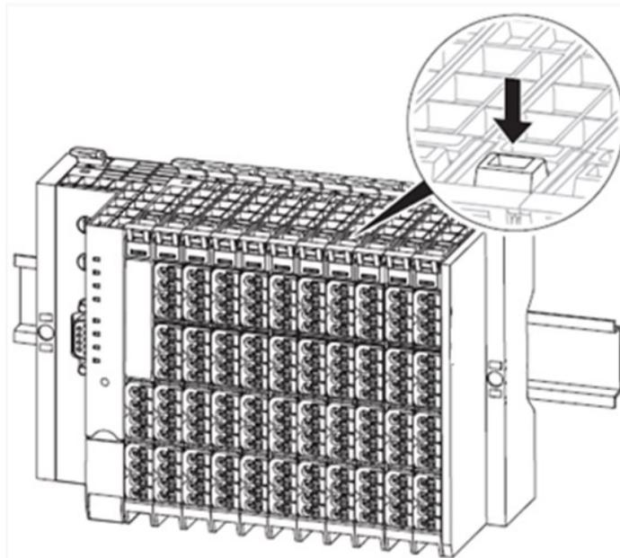
2. Press both sides of the connector together so that it can be slid off the frame.
