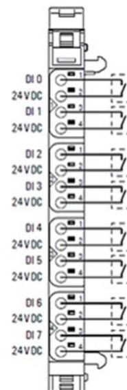
The digital input module EP-1218 can detect up to 8 input signals. Two sensors can be connected to each connector using a 2-wire connection. A status LED is assigned to each channel. The module electronics supply the connected sensors with power from the input current path (IIN).
