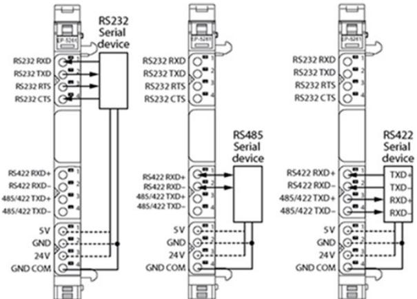
Serial data can be exchanged between the PLC and a data terminal device using the EP-5261 communication module. The device (such as a barcode scanner, printer) can be connected through an interface type RS232, RS485 or RS422.
