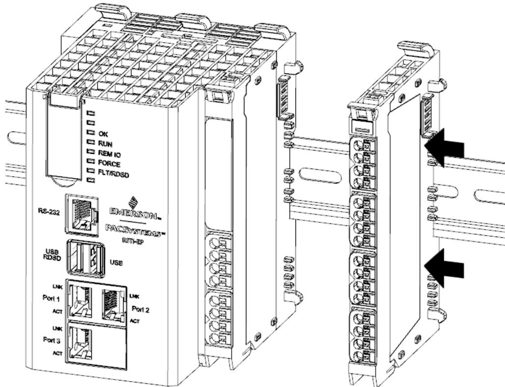
3. After all the I/O modules have been connected, mount the protective endplate into the last I/O module to protect the exposed connectors.
