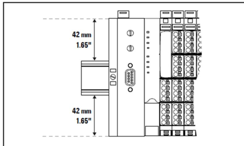
Installation on vertically positioned DIN rails is also possible. In this event, however, the heat dissipation is reduced such that the derating values change (refer to Section, Current Demand and Power Supply).
