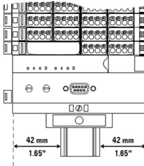
A RSTi-EP station may only be installed in this sequence (starting from the left/bottom):
