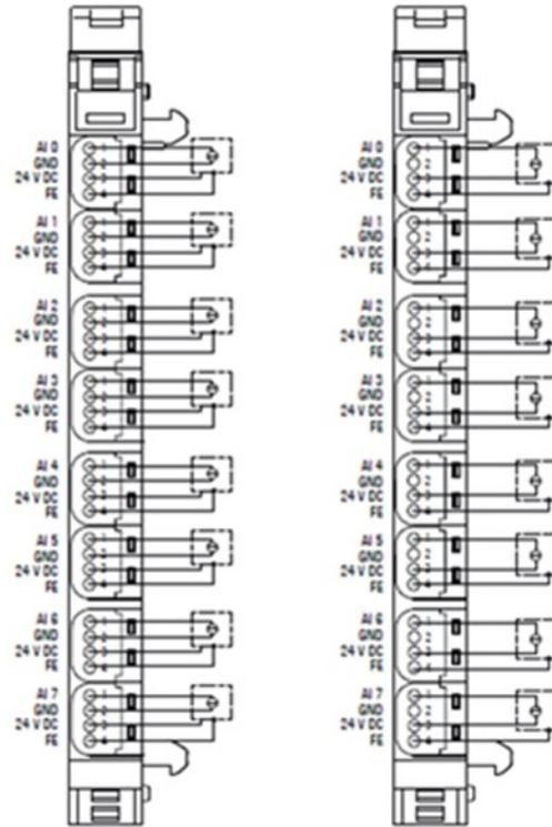
The analog input module EP-3368 can detect up to 8 analog sensors with 0-20 mA or 4-20 mA. The resolution is 16 bits per channel. Sensors can be connected to each connector in a 2-wire, 3-wire or 3-wire connection + FE (IDC). The measurement range is defined using parameterization. A status LED is assigned to each channel. The module electronics supply the connected sensors with power from the input current path (IIN).
