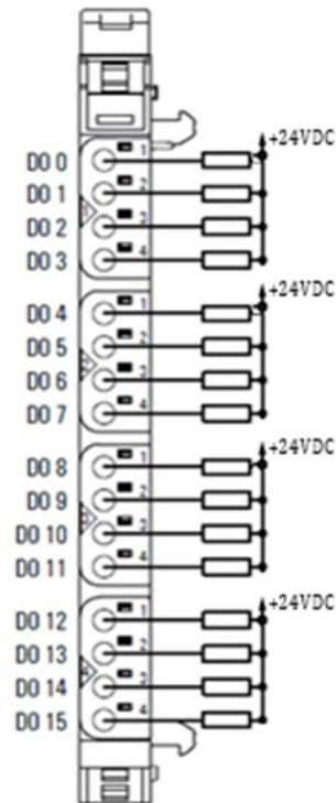
The EP-291F digital output module can control up to 16 discrete outputs, each with a maximum of 0.5 A. Four discrete outputs can be connected to each connector. The outputs are N-Switching. A status LED is assigned to each channel. The outputs are supplied with power from the output current path (IOUT).
