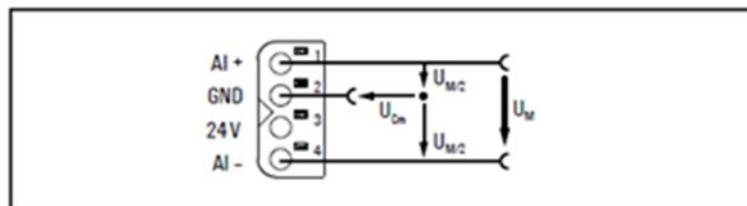
The EP-3664 analog input module can record up to 4 analog sensors with  $\pm 10V$ ,  $\pm 5V$ , 0-10V, 0-5V, 2-10V, 1-5V, 0-20mA or 4-20mA. The resolution is 16 bits per channel. Sensors can be connected to each connector in a 2-wire, 3-wire or 4-wire connection. The measurement range is defined using parameterization. Two status LED are assigned to each channel. The module electronics supply the connected sensors with power from the input current path (IIN).
