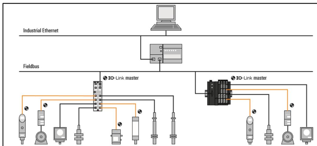
IO-Link is a communication protocol for automation technology. IO-Link enables serial, bi-directional point-to-point communication between devices on the sensor-actuator level and devices on the field level or control level. Besides cyclic process data, IO-Link allows parameters, diagnoses and identification data to be exchanged acyclically. IO-Link is standardized worldwide in IEC 61131-9 under the designation "single-drop communication interface for small sensors and actuators" (SDCI).
