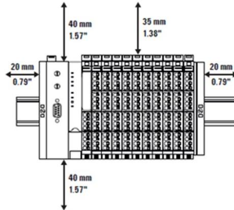
**Figure 13: Clearances for Vertical Installation**
