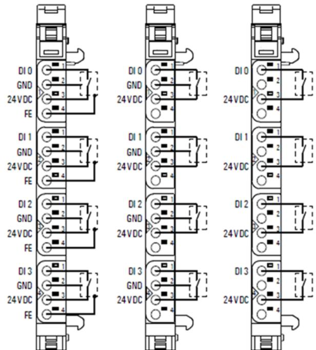
The digital input module EP-1214 can detect up to 4 input signals. One sensor can be connected to each connector using a 2-wire, 3-wire or 3-wire + FE connection. A status LED is assigned to each channel. The module electronics supply the connected sensors with power from the input current path (IIN).
