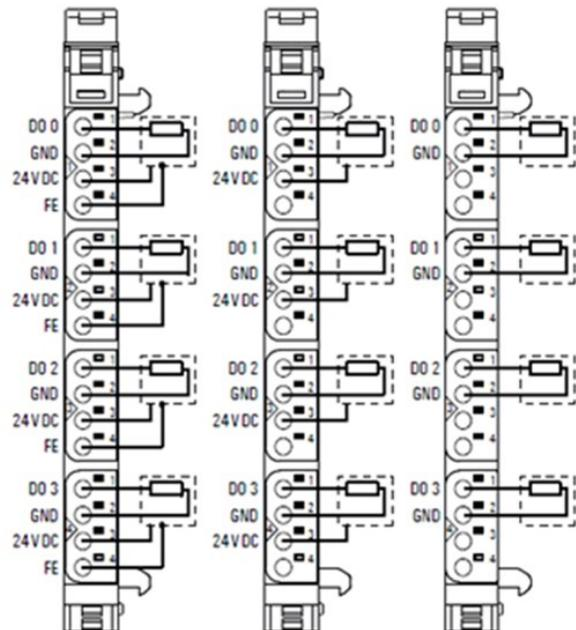
The digital output module EP-2614 can control up to 4 discrete outputs, each with a maximum of 2 A. One discrete output can be connected to each connector using a 2-wire, 3-wire or 3-wire connection + FE. A status LED is assigned to each channel. The outputs are supplied with power from the output current path (IOUT).
