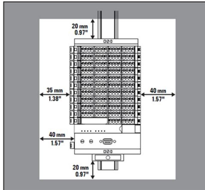
**Figure 288: Minimum Distance to Switch Cabinet Door (with/without Swivel)**
