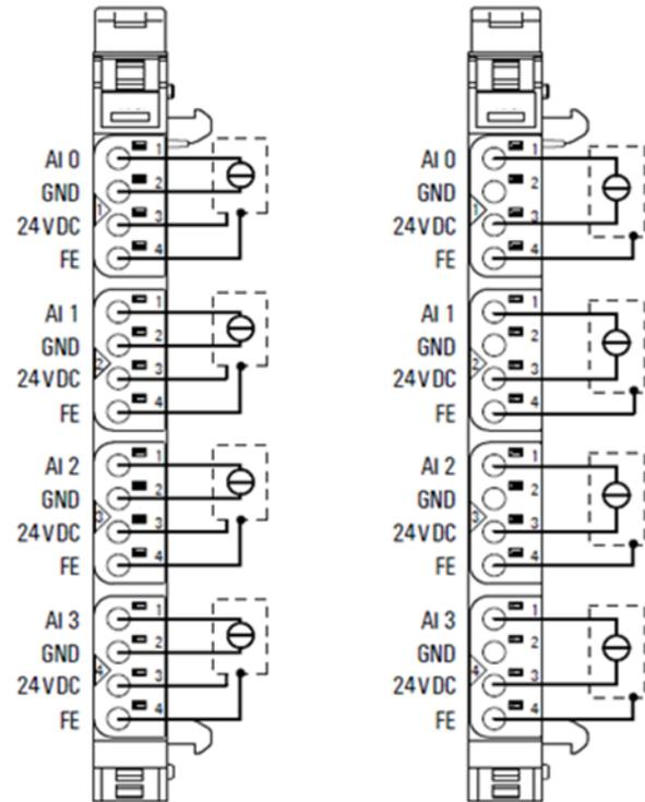
left: 3-wire sensor with sensor wiring via electronics.
