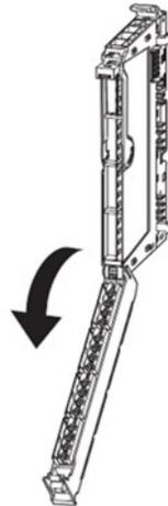
2. Lift the electronic unit removal lever and swivel it forwards by 90°.
