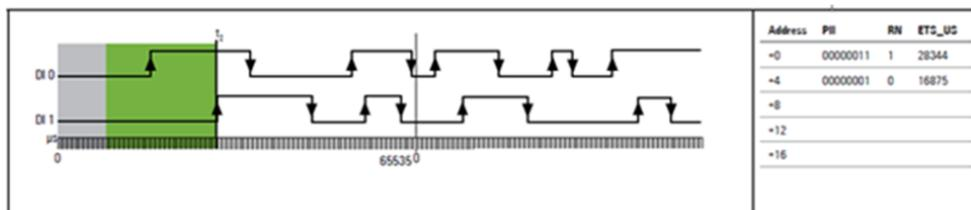
A falling 1-0 edge on DI 0 causes the 3rd ETS entry.
