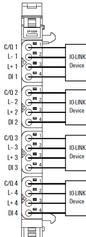
The EP-5324 module is an IO-Link master according to the IO-Link specification V1.1.2. One IO-Link device can be connected to each connector. The IO-Link devices must conform to port class A. Port class B is also possible if additionally, potential distribution modules are used. One digital input can be used additionally with each connector.
