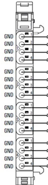
The potential distribution module EP-710F provides 16 connections for ground from the input current path. Potential distribution modules are passive modules without fieldbus communication, therefore they are not considered during configuration.
