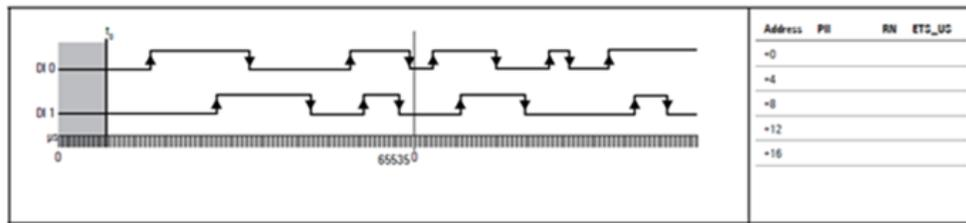
A rising 0-1 edge on DI 0 causes the 1st ETS entry at address + 0.
