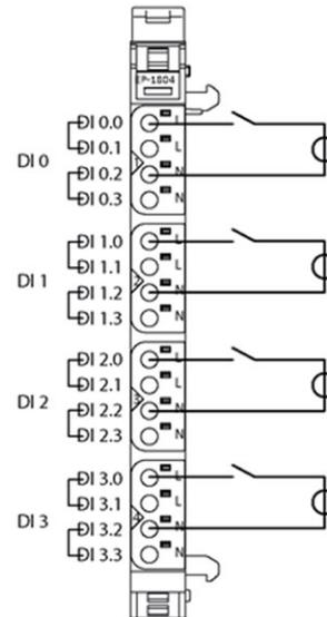
The digital input module EP-1804 can detect up to 4 binary control signals. One sensor can be connected to each connector using a 2-wire connection. Both L and N connections of each input are bridged internally. The four inputs are galvanic isolated, they can be supplied with input voltages between 110Vac and 230Vac. Solely AC measurements can be run.
