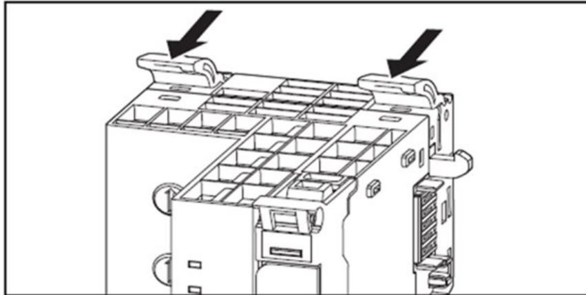
5. Place the field bus network adapter (module side to the right) on the DIN rail so that it audibly clicks into place.
