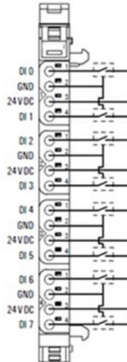
The digital input module EP-1318 can detect up to 8 input signals. Two sensors can be connected to each connector using a 2-wire or 3-wire connection. A status LED is assigned to each channel. The module electronics supply the connected sensors with power from the input current path (IIN).
