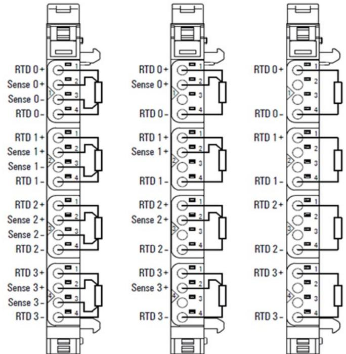
The analog input module EP-3704 can detect up to 4 analog resistance thermometers. The resolution is 16 bits per channel. A sensor can be connected to each connector in a 2-wire, 3-wire or 4-wire connection. Mixed operation using different sensors as well as different connection methods is possible. Sensor type and temperature range are set using parameterization. A status LED is assigned to each channel.
