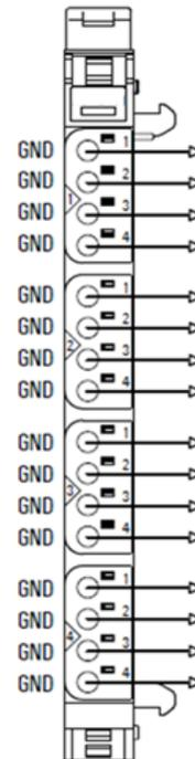
The potential distribution module EP-750F provides 16 connections for ground from the output current path. Potential distribution modules are passive modules without fieldbus communication, therefore they are not considered during configuration.
