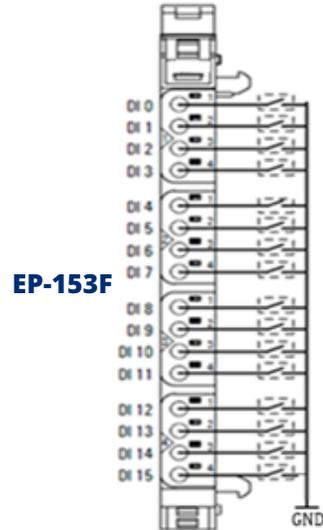
The EP-153F digital input module can detect up to 16 input signals. Four sensors can be connected to each connector in a 1-wire connection. A status LED is assigned to each channel. The connected sensors must be supplied with power from the input current path IIN (e.g. with potential distribution modules).
