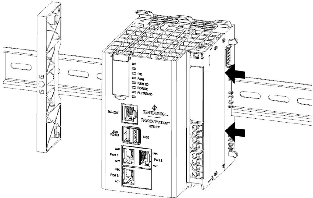
2. Repeat the steps for each of the IO modules. Connect the first IO module into connectors on the right side of the controller. Each subsequent IO module will connect to the previous module.
