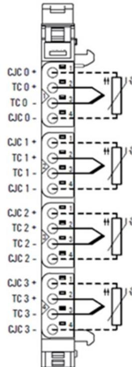
The analog input module EP-3804 can detect up to 4 analog thermocouple sensors or voltages between  $\pm 15$  mV and  $\pm 2$ V. The resolution is 16 bits per channel. Sensor type and temperature range are set using parameterization. Mixed operation using different sensors is possible. For each channel, an internal or external cold-junction compensation (CJC) can be parameterized. A status LED is assigned to each channel.
