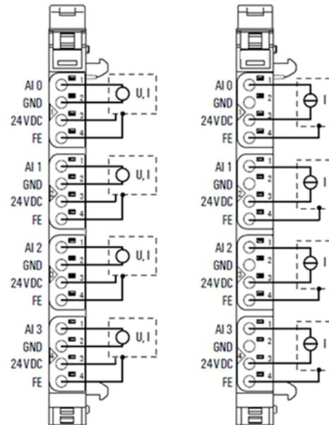
left: 3-wire sensor with sensor wiring via electronics.
