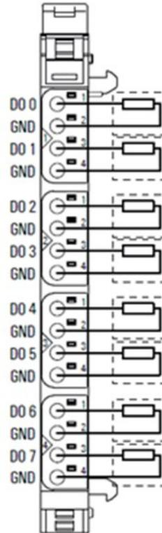
The EP-2218 digital output module can control up to 8 discrete outputs, each with a maximum of 0.5A. Discrete outputs can be connected to each connector in a 2-wire connection. A status LED is assigned to each channel. The outputs are supplied with power from the output current path (IOUT).
