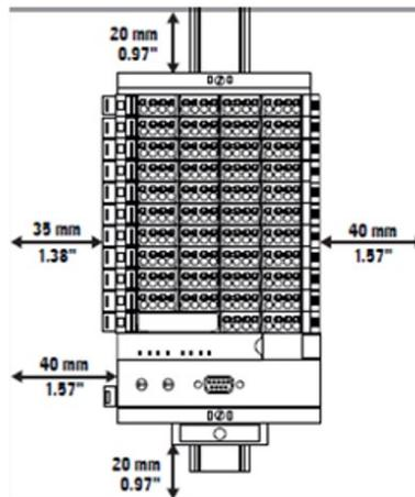
**Figure 14: Clearances for Electrical Cabinet Door (Without/With Swivel Marker)**
