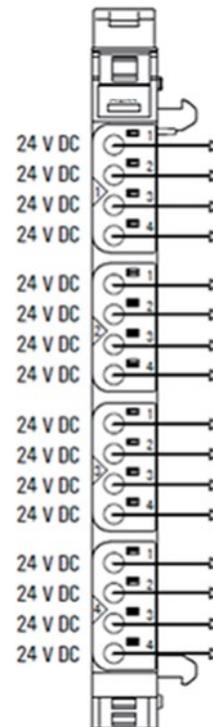
The potential distribution module EP-751F provides 16 connections for +24 V from the output current path. Potential distribution modules are
