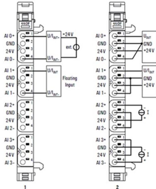
(Figure 209: For EP-3664, the 1= Standard, 2= Alternative option)
