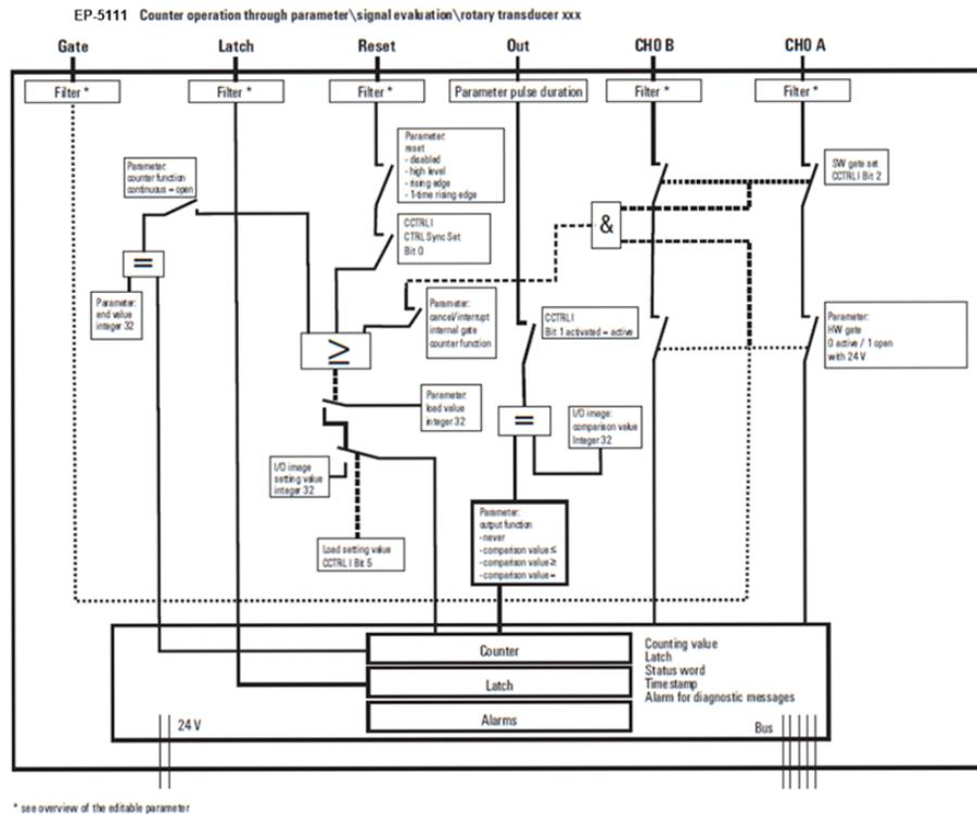
**Figure 144: EP-5111 Counter Operation using Pulse/Direction (A/B)**
