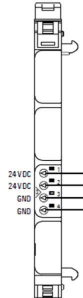
Power-feed modules are used to refresh the current paths and isolate the power supply. The main power supply of the RSTi-EP station is always fed in via the network adapter. A power-feed module EP-7631 must be connected if the current demand of the series of input modules is too large.
