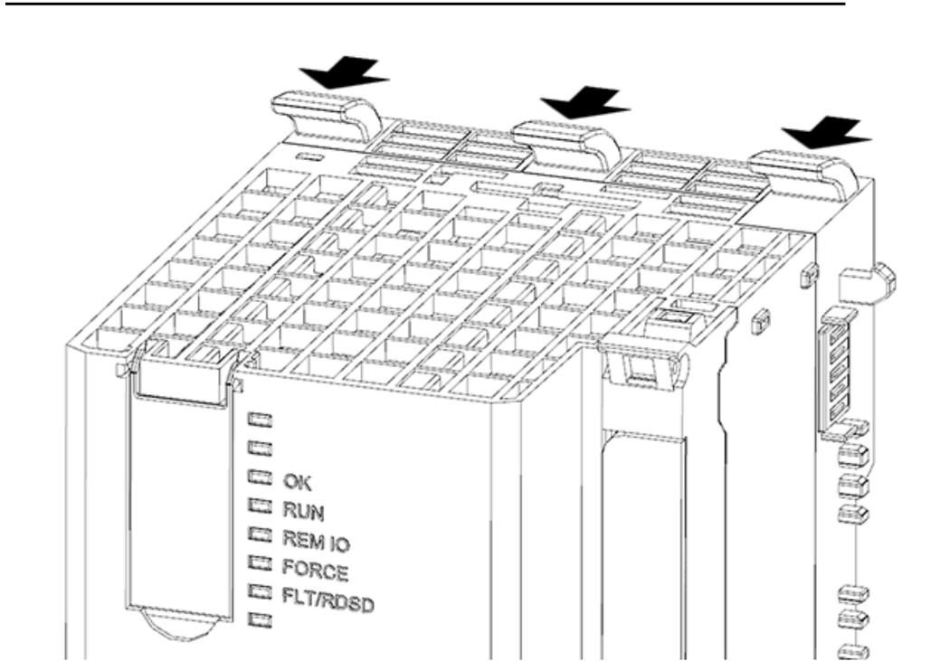
2. Attach the controller to the DIN rail. The controller should rest on the rail, but be able to move freely side-to-side.
