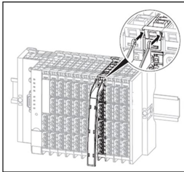
16. Insert the labelled marker into the swivel marker from below.
