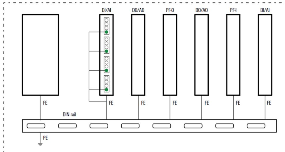
The spring contacts underneath the module and the network adapter snap into the DIN rail to make a connection.
