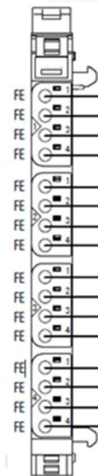
The potential distribution module EP-700F provides 16 connections for the functional earth. Potential distribution modules are passive modules without fieldbus communication, therefore they are not considered during configuration.
