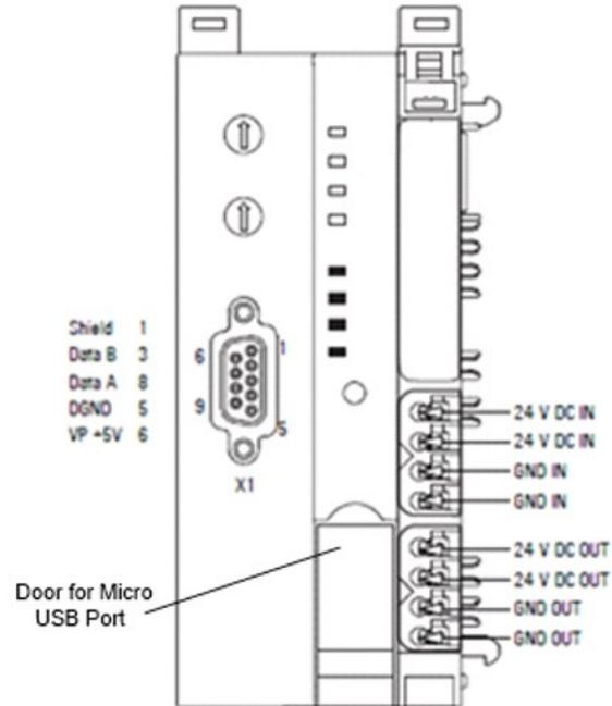
**Figure 23: Block Diagram EPXPBS001**
