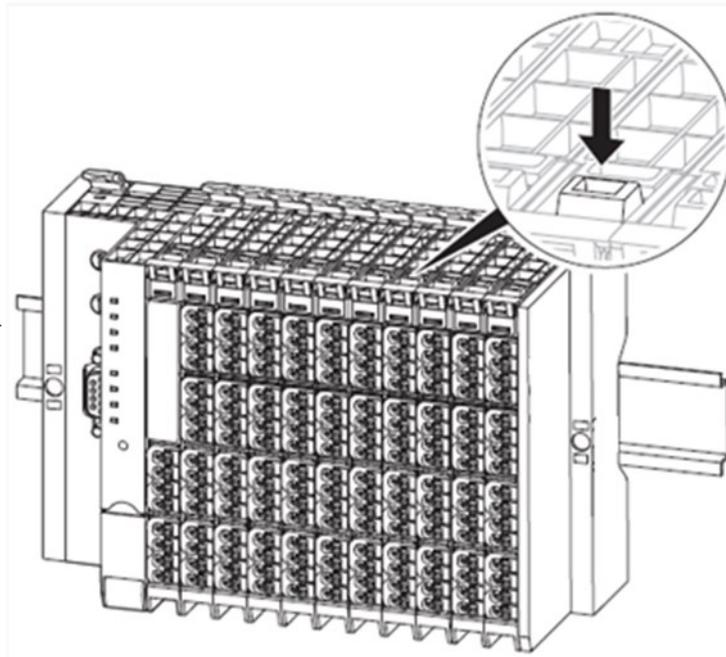
2. Swivel the plug-in unit with the cabling towards the front by 90°.
