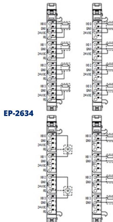
The digital output module EP-2634 can control up to 4 discrete outputs each with a maximum of 2 A. One discrete output can be connected to each connector in a 2-wire or 3-wire + FE connection. A status LED is assigned to each channel. The outputs are supplied with power from the output current path (IOUT).
