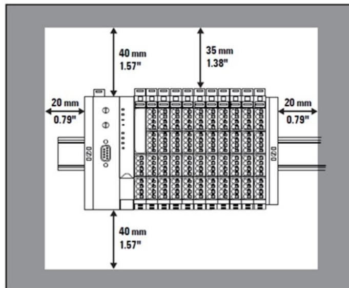
**Figure 287: Clearances with Vertical Installation**
