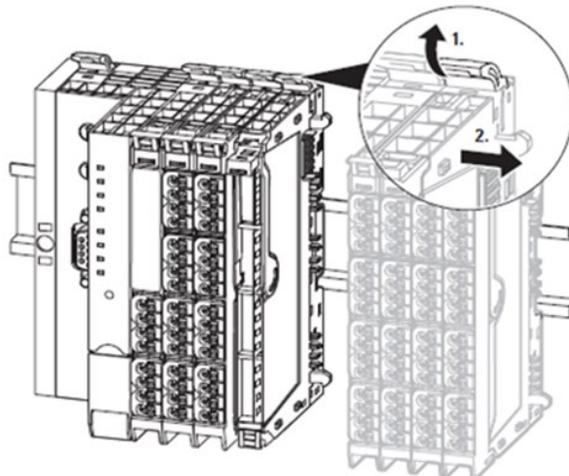
8. Slide the module to the right and remove it from the DIN rail.
