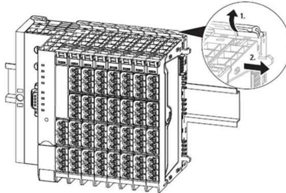
4. Slide the module on the DIN rail approximately 5 cm (2 in) to the right, push it onto the DIN rail and click the release lever into place.
