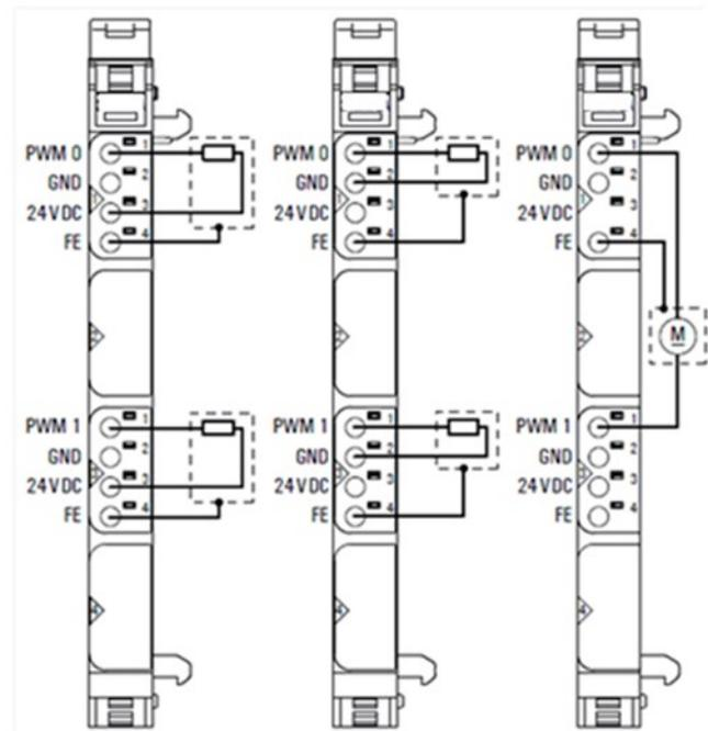
The digital pulse width modulation modules EP-5442 is used for the control of small motors with current requirements of up to 2 A. The period duration for each channel can be parameterized from 25µs to
