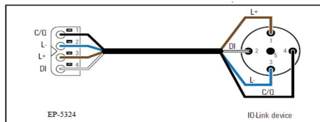
**Note:** The use of the additional digital input at the DI connection is optional. It can be used as digital input, e.g. if the IO-Link device provides an additional switching signal.
