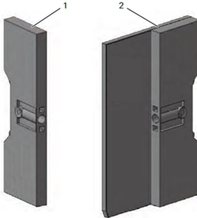
Each RSTI-EP fieldbus network adapter is delivered together with a termination kit EP-8301. This comprises two end brackets and an end plate. The end plate protects the contacts on the last module at the end of the RSTI-EP station. The station is fixed to the DIN rail on both sides via the end brackets.
