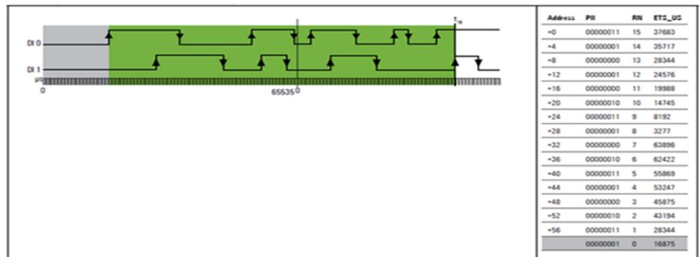
A falling 1-0 edge on DI 1 causes the 17th ETS entry. The 2nd ETS entry is deleted and not available anymore.
