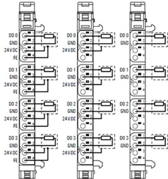
The EP-2214 digital output module can control up to 4 discrete outputs, each with a maximum of 0.5 A. One discrete output can be connected to each connector using a 2-wire, 3-wire or 3-wire connection + FE. A status LED is assigned to each channel. The outputs are supplied with power from the output current path (IOUT).
