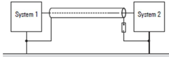
For longer lengths of shielded cables, such as if a sensor must be added to a control panel, a potential difference between both end points must not be ignored.
