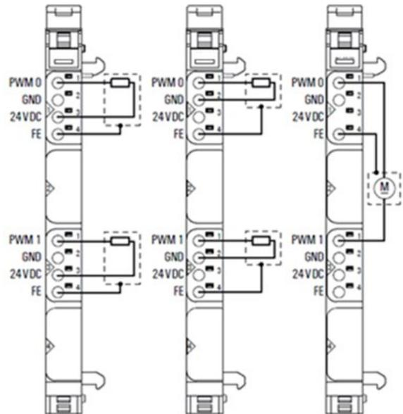
The digital pulse width modulation module EP-5422 is used for the control of small motors with current requirements of up to 0.5 A. The period duration for each channel can be parameterized from 25 $\mu$ s to approx. 175ms (input values from 1,202 to 8,388,607 based on a factor 0.02083 $\mu$ s).
