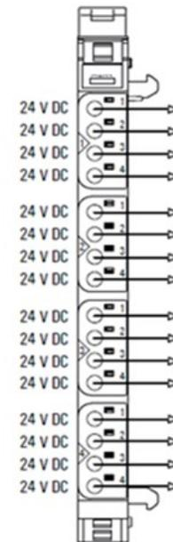
The potential distribution module EP-711F provides 16 connections for +24 V from the input current path. Potential distribution modules are passive modules without fieldbus communication, therefore they are not considered during configuration.
