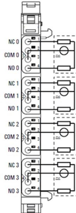
The digital relay output module EP-2714 can control up to 4 discrete outputs, each with a maximum of 6A. Each connector features a potential-free changeover contact. The relay coils are supplied with power from the output current path ( $I_{OUT}$ ).
