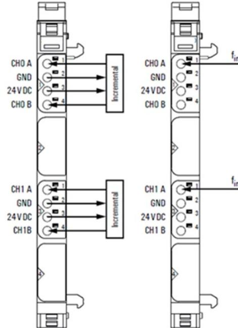
The digital counter module EP-5112 can read square-wave signals (for example, from an incremental encoder) with a maximum input frequency of 100 kHz. Depending on the operating mode, both 32-bit counters can count up/down independent of each other in a preset range of values. The counters can be controlled via software by setting the appropriate control word.
