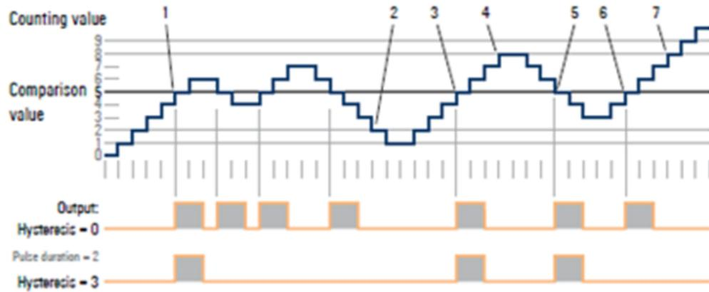
1. Comparison condition met → pulse of the parameterized duration is output, hysteresis activated
