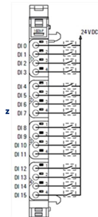
The EP-125F digital input module can detect up to 16 input signals. Four sensors can be connected to each connector in a 1-wire connection. A status LED is assigned to each channel. The connected sensors must be supplied with power from the input current path IIN (e.g. with potential distribution modules).
