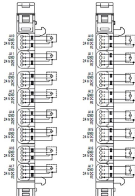
The analog input module EP-3468 can detect up to 8 analog sensors with 0-20 mA or 4-20 mA. The resolution is 16 bits per channel. Sensors can be connected to each connector in a 2-wire, 3-wire or 3-wire connection + FE (IDC). The measurement range is defined using parameterization. A status LED is assigned to each channel. The module electronics supply the connected sensors with power from the input current path (IIN).
