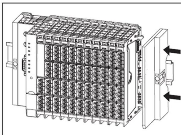
13. Screw down the end bracket tightly (using a 3-mm screwdriver).
