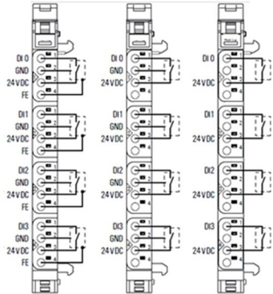
The digital input module with time stamp functionality EP-12F4 can detect up to 4 binary control signals and provide them with a time stamp (resolution 1 $\mu$ s). Depending on the configuration of the module, up to 5 or 15 time-stamp entries can be evaluated.
