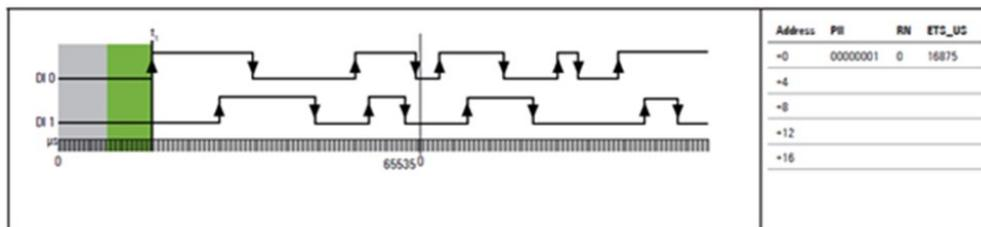
A rising 0-1 edge on DI 1 causes the 2nd ETS entry at address + 0. The 1st ETS entry is shifted by 4 bytes.
