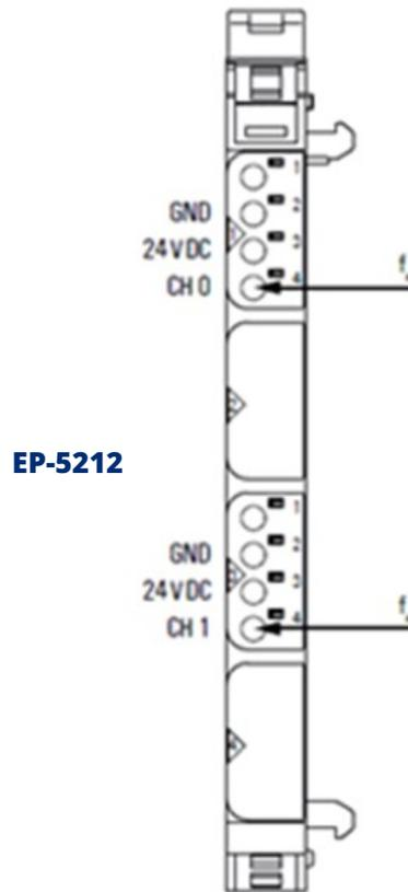
The digital counter module EP-5212 can read frequency of one square-wave signal (1 channel) from one or two external sensors with a maximum input frequency of 100 kHz. Frequencies to be counted are applied to channel CH0 and/or channel CH1, the measurement will be started via control word 1 and 2 respectively. Measuring cycles can be defined in  $\mu\text{s}$ . The longer the measuring cycle the more exactly the measurement.
