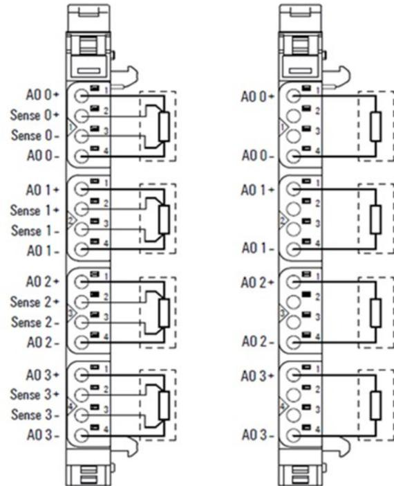
The analog output module EP-4164 can control up to four analog actuators with  $\pm 10V$ ,  $\pm 5V$ , 0-10V, 0-5V, 2-10V, 1-5 V, 0-20 mA or 4-20 mA. The resolution is 16 bits per channel. An output can be connected to each connector, the internal switching is carried out automatically. The output range is defined using parameterization. A status LED is assigned to each channel. The outputs are supplied with power from the output current path (IOUT).
