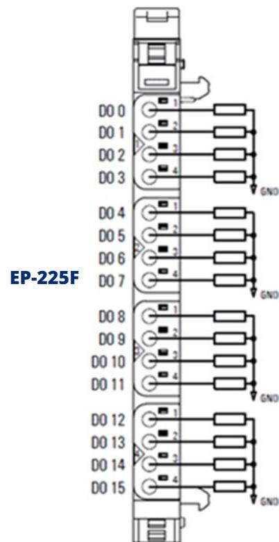
The EP-225F digital output module can control up to 16 discrete outputs, each with a maximum of 0.5 A. Four discrete outputs can be connected to each connector. A status LED is assigned to each channel. The outputs are supplied with power from the output current path (IOUT).
