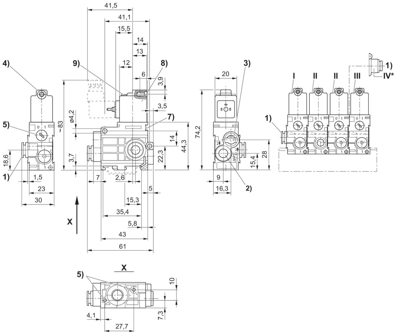
1) Port 1 2) Port 2 3) Port 3, exhaust air must not be throttled 4) Core  $\varnothing$  for M5 5) Manual override 6) Pocket hole 6 mm deep for 3.5 self-tapping screw 7) Mounting space for name plate 8) Coil can be rotated at 180° intervals 9) LED \* Air conn. module (item IV) mounted onto stacking valve (item II) permits additional air supply from right hand side. End valve (item III) not required.
