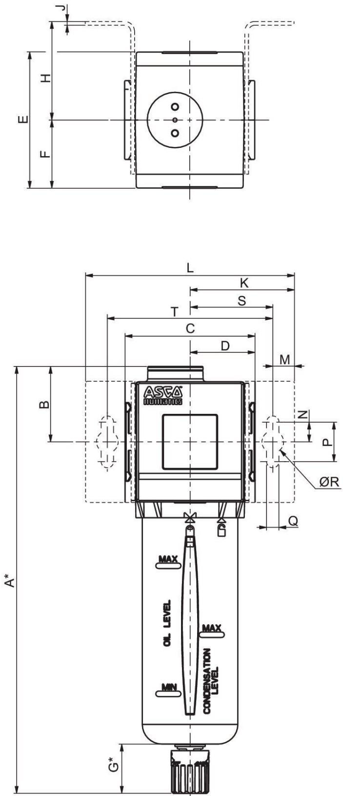
\*Variable dimension based on the type of drain specified, if an automatic drain is specified, add another [5] mm to the "G" dimension, which also adds 5 mm to the "A" dimension.
